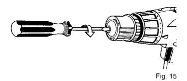
Insert hex key wrench in chuck and tighten chuck jaws securely. Tap sharply with a mallet in a counterclockwise direction. This will loosen chuck on the spindle. It can now be unscrewed by hand. See Figure 16.
